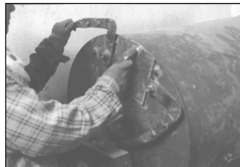
The wedge lock makes the end door easy to open and close.
