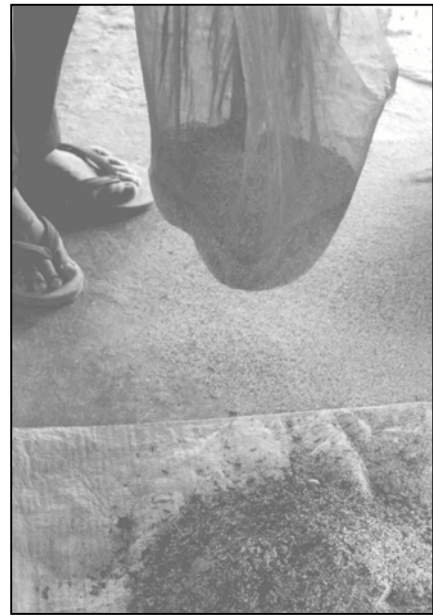
Sifting brick chips out of the ash is a dusty job.
