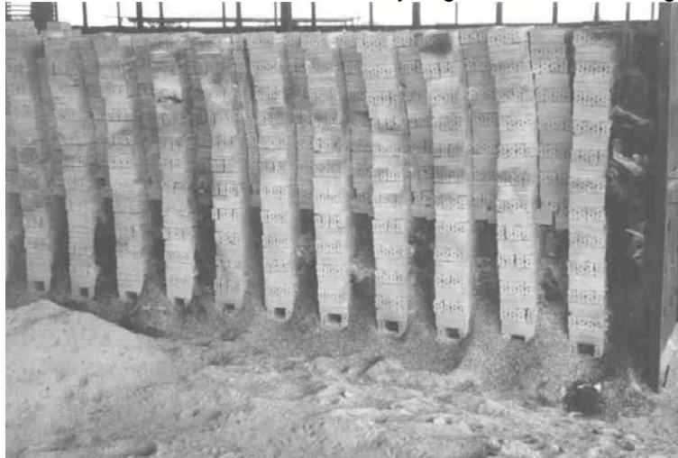
A field brick kiln fired with rice husks.
