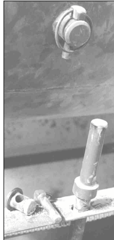
A clevis holds the lifting rods in place. Plugs with "O" rings are used when grinding.
