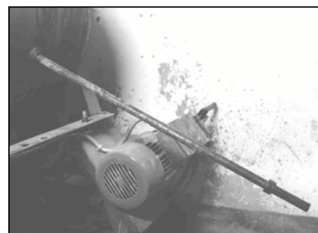
The 2 lift rods are inserted in the side of the drum. Rotating the drum raises the grinding rods for easy ash removal.
