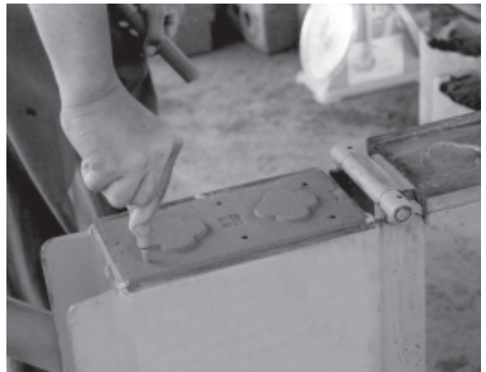
Use a penetrometer to check blocks in 6 places to make sure the density is the same.
